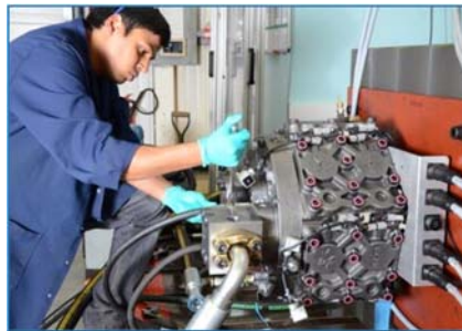
Figure 13. 480 cc/rev DD Pump/Motor ® on test stand (Artemis)
