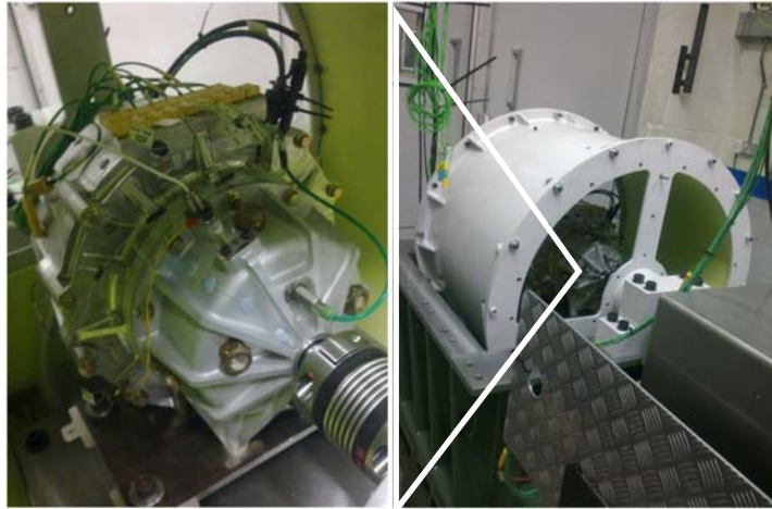
Figure 18. Flywheel module installed at Ricardo test facility
